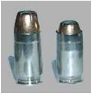
(Above) The cartridge on the left is a normal .40 S&W round. On the right is a round that was taken from an officer at a recent training session. Note the bullet has been set back into the case about 1/10th of an inch.
