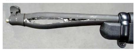
The ammunition - Sellier & Bellot, is a brand that is frequently found at discount mail order sites and not commonly used in law enforcement. As the photos show, the first round lodged in the barrel and the subsequent rounds piled up behind it until the barrel failed under the pressure of the .40 S&W load.
