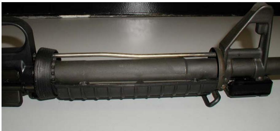
Stock AR gas system showing gas tube and associated parts
