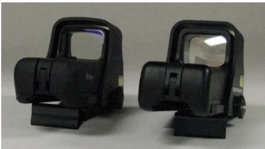
This photo shows the reflection off the optics of a genuine and a counterfeit Model 553. The difference in the amount of reflection from the two sights is easily discerned.
