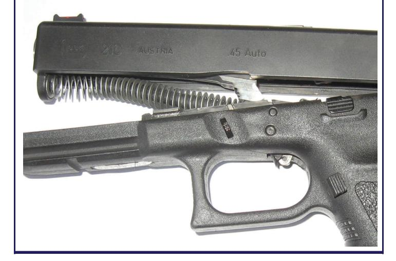
Catastrophic Pistol Failure Photos courtesy of Greg Newman
