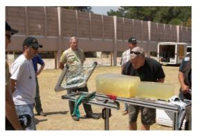
Core jacket separation is common when firing through auto glass, however Federal's HST round did not shed its jacket and expanded 22% larger than Winchester's SXT and 40% larger than Winchester's JHP. The HST also retained 26% more weight than the SXT.
