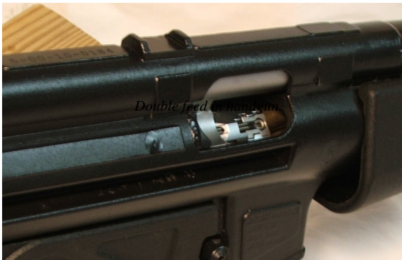
Double feed in a HK MP5. Note how difficult it is to see into the chamber on this type of weapon..
