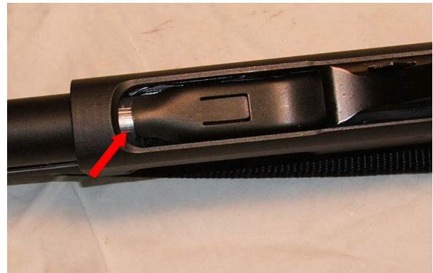
Double feed in a Remington 870 pump shotgun. Note the shell between the carrier and bolt.
