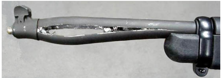
First round fired in this Ruger PC4 carbine became lodged in the barrel due to a squib round. The shooter failed to note the reduced recoil and lack of muzzle report. After performing an immediate action drill, several more rounds were fired resulting in this catastrophic failure of the weapon.
