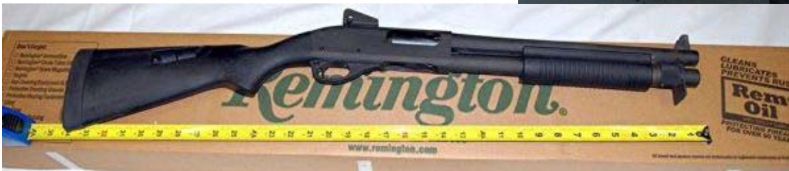
Remington 870 U.S. Secret Service model (above) and Mossberg 590 (left) fitted with a 14 inch barrel, Speed feed stock and Ghost Ring sights.
